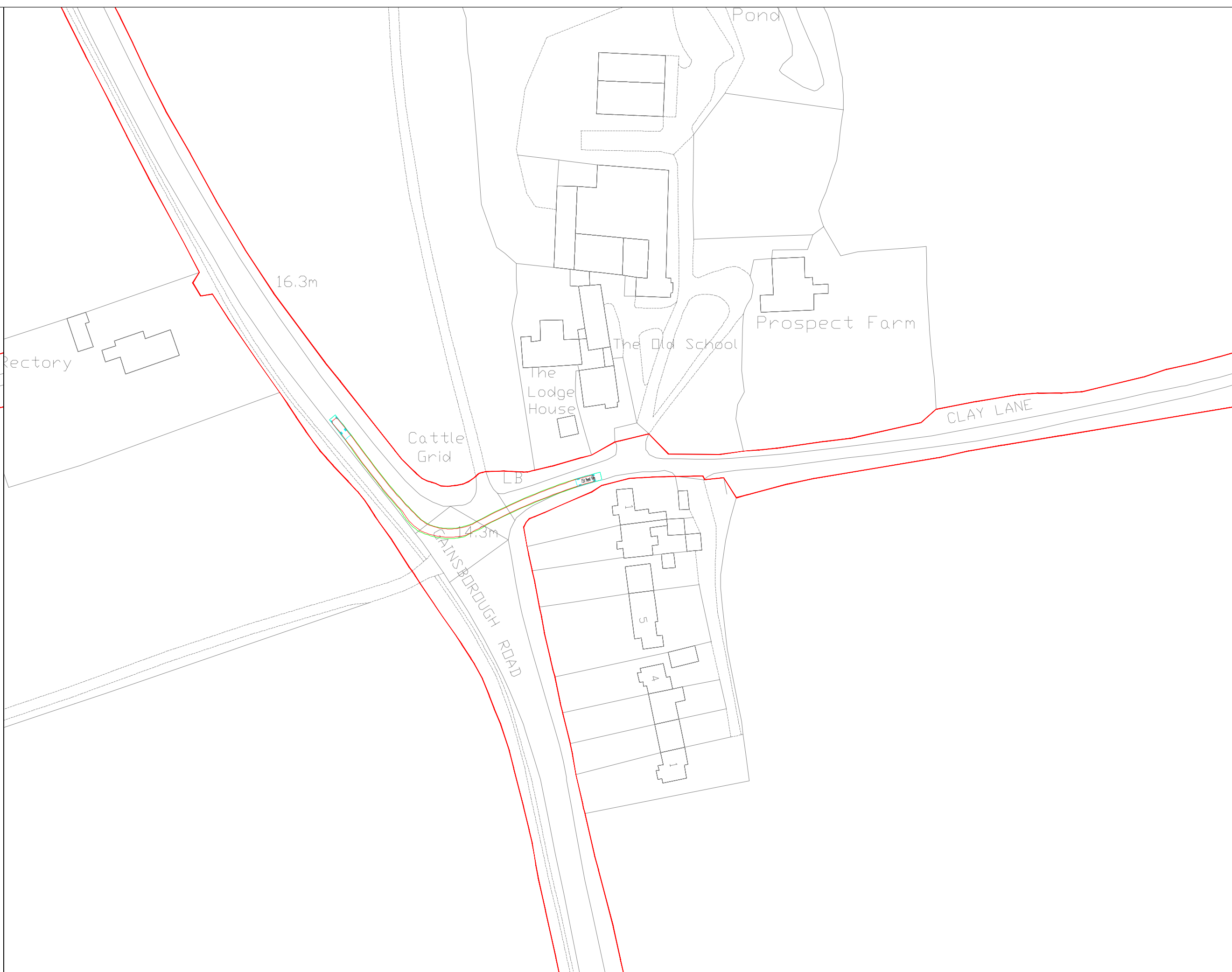
7.5t PANEL VAN VEHICLE MANOUVRE, HEADING WEST OUT OF CLAY LANE TURNING RIGHT ONTO ON GAINSBOROUGH ROAD A156 HEADING NORTH - SCALE 1:1000
